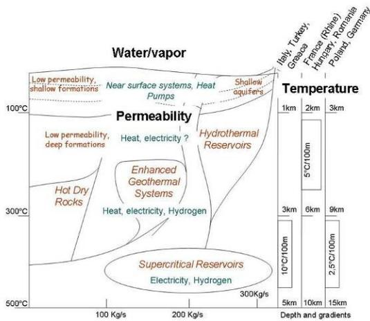
Figure 1: Sketch vision of the geothermal resources
