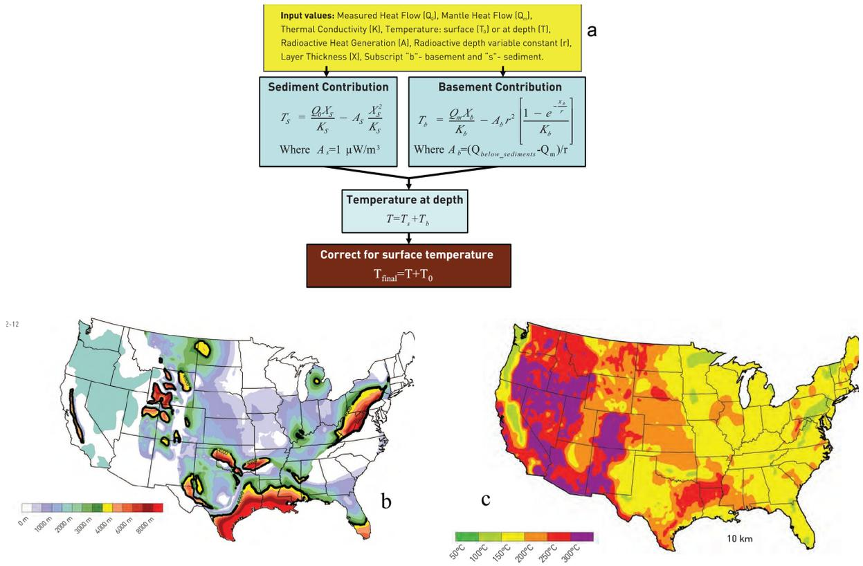
Figure 3: Calculation of temperature at depth in US (The future of Geothermal Energy, 2006). a: Flow chart for calculation of temperature at depth; b: Average thickness of sediments; c: Average temperature at 10 Km depth
