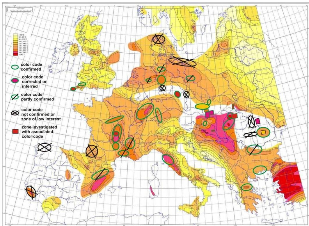
Figure 4: Map of the temperatures extrapolated at 5km depth as inferred from twenty to thirty years old individual maps, and validation of anomalously hot zones as revealed by a recent revision (Genter et al., 2003). The Rhine graben anomaly is clearly validated.
